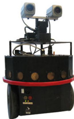
Figure 26: Athos is a two-wheeled robot equipped with a pan and tilt stereo head.
