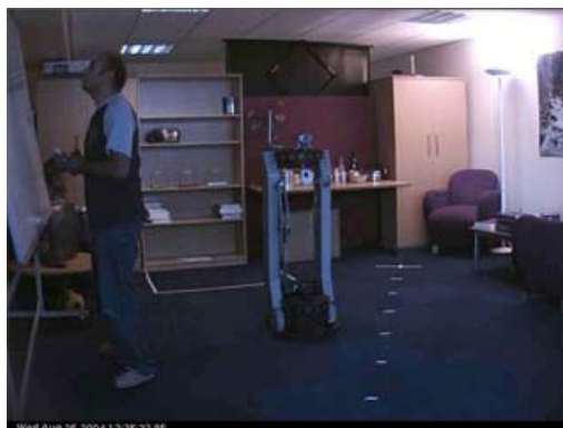
Fig. 9 Illustration of the phantom effect: uncomfortable data was recorded by the Comfort Level Device when a subject opened a whiteboard pen with both hands while still holding the Comfort Level Device in one hand.
