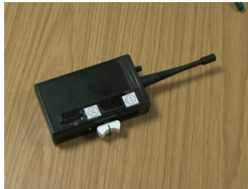
Figure 21: Comfort Level Device to allow subjects to indicate their comfort levels during HRI trials.
