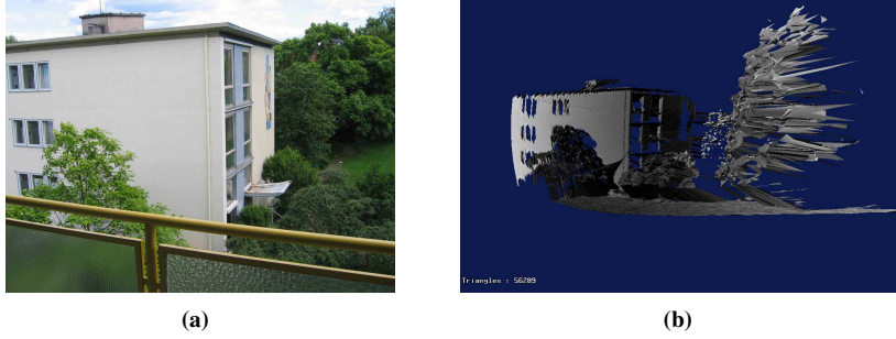
Figure 2. Sample with 80m range (original left, triangulated point cloud right)
