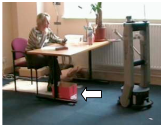
Fig. 2: A subject sitting at the desk, showing a box placed under the table to create a target for the robot's sonar sensors.
