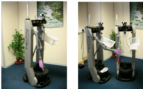
Fig. 1: The PeopleBot™ robots fitted with a pointer (in raised and lowered positions) and basket.
