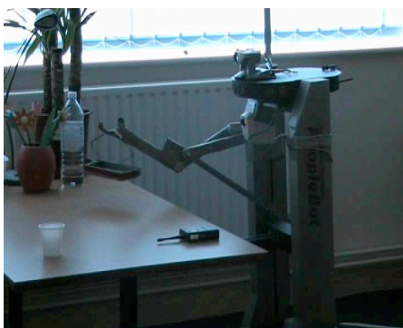
Fig. 4: The robot, fitted with a hook-like end-effector, was able to fetch small items in special pallets.
