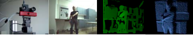
Fig. 1. Sensor head (left), 2d image (middle left), disparity image (middle right), 3d image (right)
