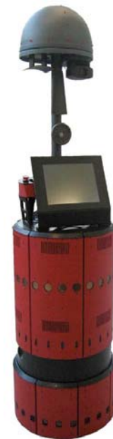
Rackham is an interactive robot able to interact with humans and guide them on an exhibition.
