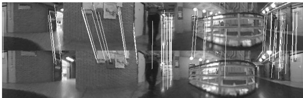
Figure 6: A panoramic image, annotated with positions of extracted SIFT features. Arrows indicate the scale and main orientation of the feature.
