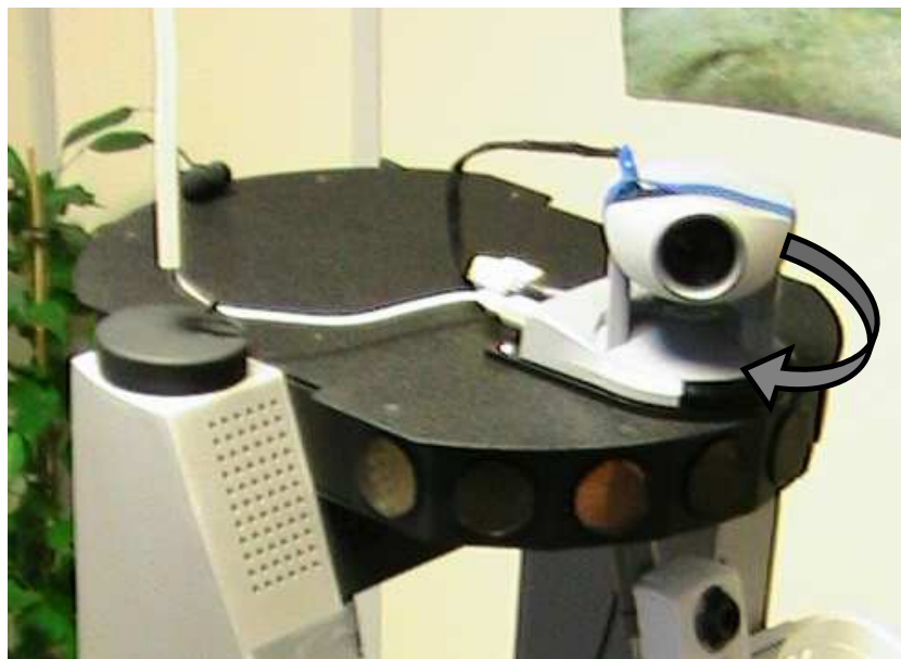
Figure 2: Detail of PeopleBot Camera. Arrow indicates panning movement by camera.
