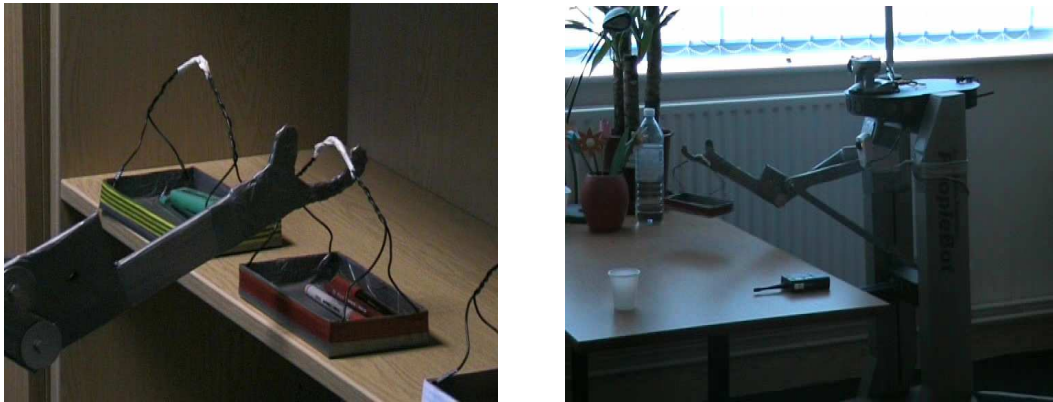
Figure 33: Details of the Robot's End-Effector and Pen Baskets. These were used for fetching required pens for the subject.
